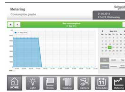
Energy metering: measure gas, water and electricity consumption
