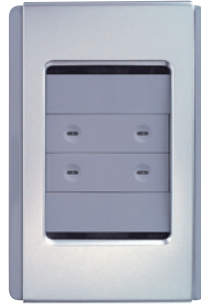
5854R8F1AA C-Bus Wireless Wall Switch, 4-Button, 1-Channel Relay, 8A (Fluorescent) Rating
