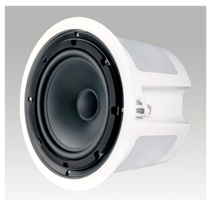
The Krix Stratospherix employs a large 8" bass driver with a concentric professional grade compression tweeter. The dual concentric driver configuration ensures uniform sound coverage in all directions. The grille is corrosion resistant Aluminium and all other hardware is stainless steel ensuring reliable performance both indoors or outdoors.
