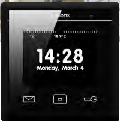
Screen saver: time, date, room temperature
