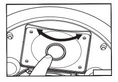
If the grille and speaker frame require painting, be sure to mask off the speaker drivers. When painting the grille, it might be necessary to thin down the paint to avoid blocking the holes in the grille. After the paint is completely dry, fit the grille to the front of the speaker.
